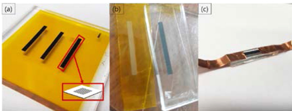
Fig. 3. (a) Carbon is generated on Polyimide (b) Generated carbon of polyimide was transferred to PDMS (c) Sensor completed with copper tape.
